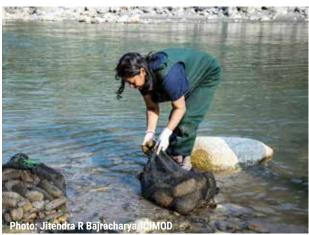
Photo 13: A researcher prepares an artificial substrate sampler to place them in an appropriate location along the bank of the watercourse. The artificial substrate sampler consists of a polyethylene netting bag filled with mineral substrates of different sizes.
