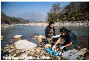
Photo 26: The researcher is measuring the water quality parameters (Nitrate, Phosphate, Ammonia) using a Hanna probe.
