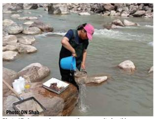
Photo 17: A researcher passes the composite benthic macroinvertebrate sample through a circular hand net with a 500 µm mesh, leaving only heavy mineral sediments at the bottom of the bucket.
