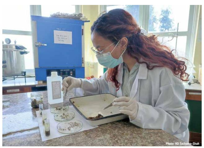
Photo 21: Sorting of macroinvertebrates from the sediments and preserved in a plastic vials with ethanol in the laboratory
