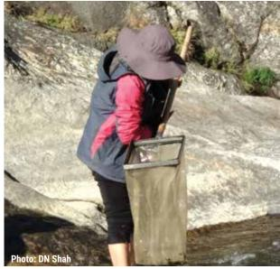
Photo 12: Sampling gear for collecting benthic macroinvertebrate samples
