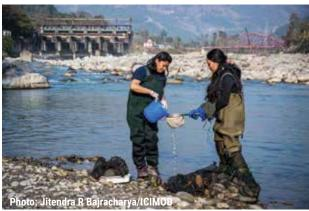
Photo 16: Researchers sieve the benthic macroinvertebrate sample using a hand net with a 500 µm mesh that was retained in the bucket after cleaning the artificial substrate sampler.
