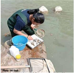
Photo 18: A researcher carefully inspects for any benthic macroinvertebrates left in the mineral substrate after passing the stirred sample through a circular hand net with a 500  $\mu$ m mesh for a few times.
