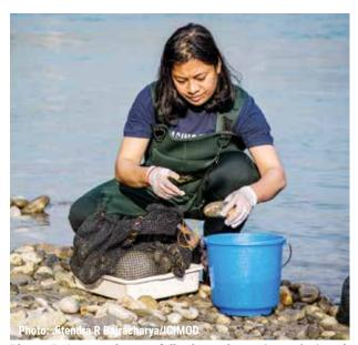
Photo 15: A researcher carefully cleans the netting and mineral substrates in a bucket half-filled with water after placing the artificial substrate sampler on the large white tray.
