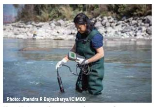
Photo 25: A researcher measures the water quality parameters (water temperature, pH, dissolved oxygen, EC, TDS, turbidity) using a Hanna probe.
